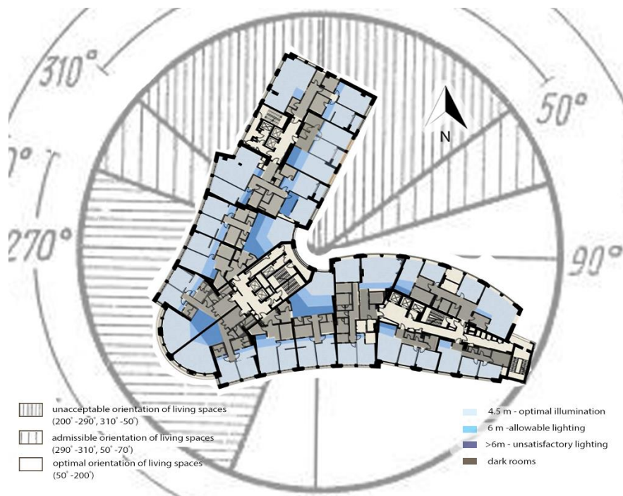
Figure 5. An analysis of the distribution of light in the premises of the Linden Luxury Residences residential complex.
